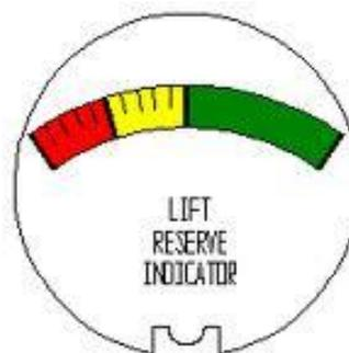
The green zone is the region where there is enough lift being produced by the wing, and the needle will most probably peg at 2.0" on the stock gauge.
