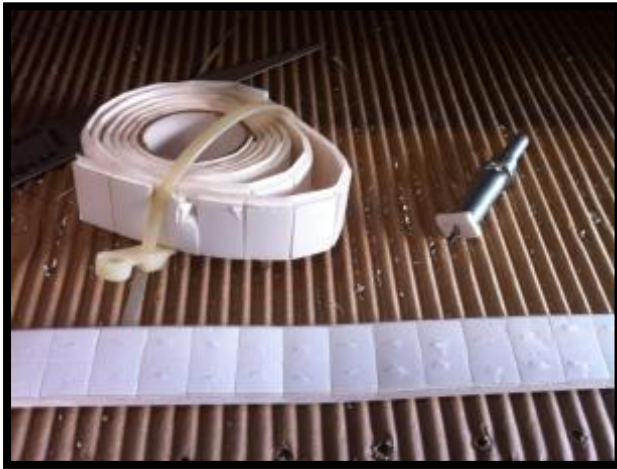
A roll of double stick pads, cut and a slit placed in the middle using a razor blade.
