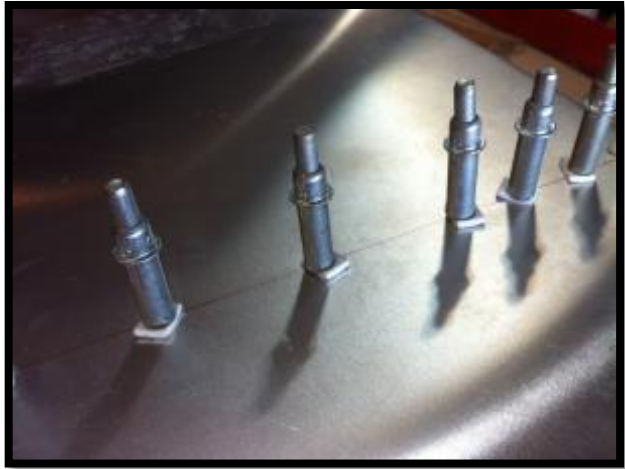
Cleco pads in action!
